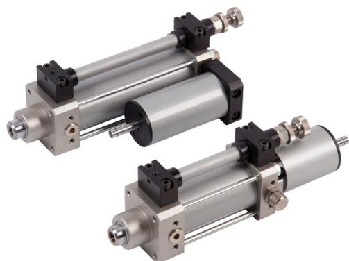
Airwork hydraulic speed regulator, is an oil system with closed circuit which has to be connected to a pneumatic cylinder in order to obtain an adjustable slowing down of the stroke.
